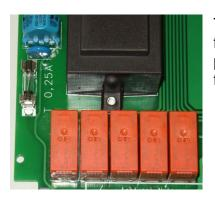
The electronic control system is protected by a 0.25A fine-wire fuse on the PCB in the inside of the device. The short-circuit protection for the filter pump must be provided by a backup fuse of maximum 16A on site.
